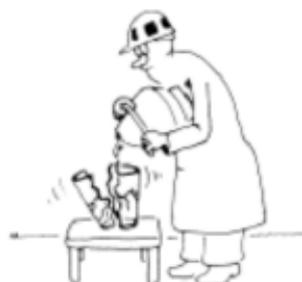
If cryogenically liquefied gases can be trapped between two valves, **pressure release systems** with a sufficiently large diameter must be provided.
