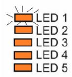
Push the **HUPE AUS/CANCEL HOOTER** button to scroll the LEDs and set the units from 1 to 9.
