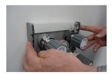
Step 5: Insert the plastic side sections into the basic profile.
