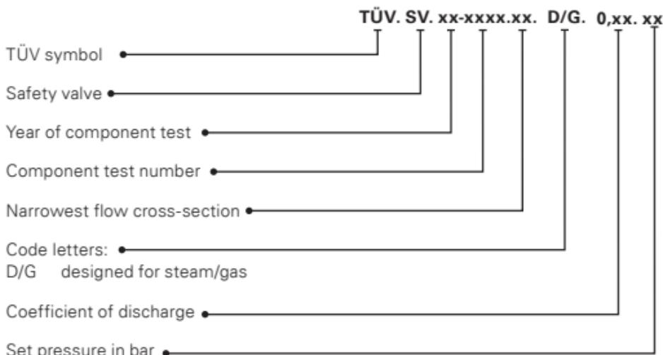
We check the safety valves for pressure resistance and tightness, adjust the requested set pressure and seal them.
